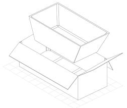
2. Place bathtub in desired location on bathroom. Attention should be given to bathtub placement to ensure the bathtub drain and plumbing are note located directly above floor joists.
